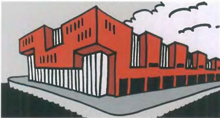
The cedar wood used in the upper part will gradually turn grey, contrasting with the terracotta colour of the prefabricated concrete walls that close the private courtyards.
