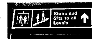
Figure 2.53 The scale of text and symbols which need to be seen from a distance is important for legibility and colour contrast of all signage
