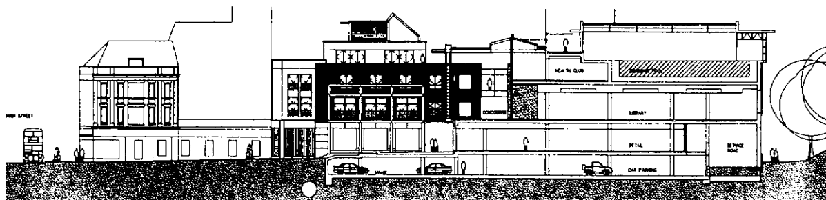
Section through Ebbisham Centre, Epsom, Surrey. The library is on the first floor (RMJM/AT)
