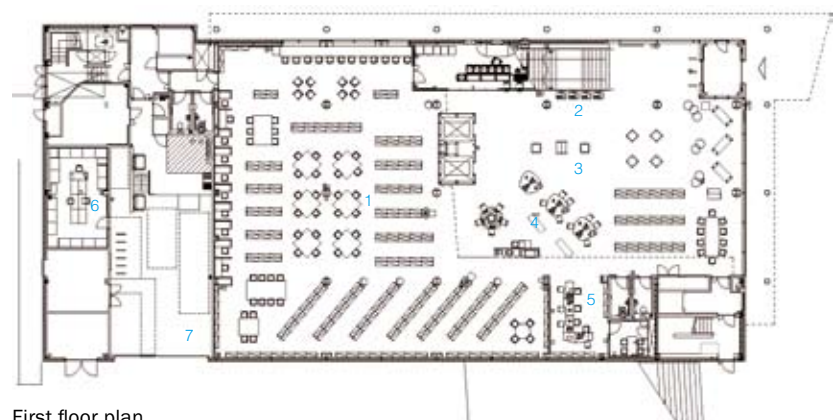
First floor plan 1. Non-fiction 2. Self service loans and returns 3. Sales 4. Information 5. Agencies 6. Dispatch 7. Service bay
