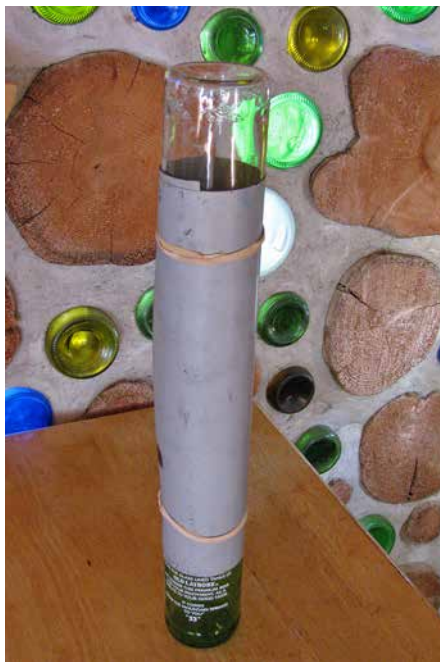
8.4. Adjusting the length of the cylinder allows for bottle-ends from 16 to 24 inches in length.
