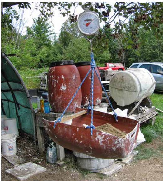
10.4. Weighing mortar materials.
