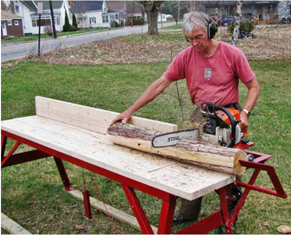
15.1. A lot of log-ends can be cut fast and accurately with this cut-off table and saw.
