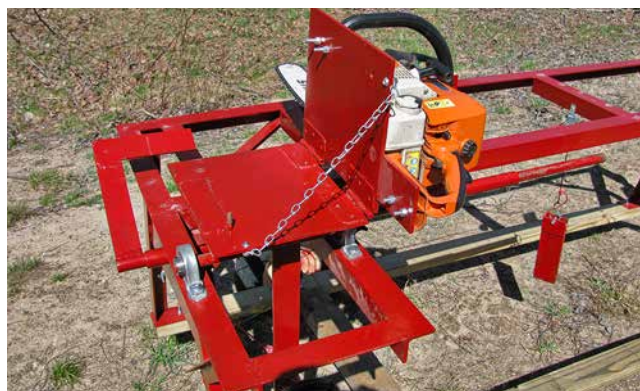
15.3. The two quarter-inch steel mounting plates are connected with two door hinges, welded to the plates. In the open position this provides access to gas and bar oil fillers.
