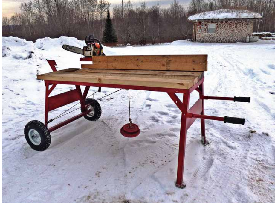
15.9. Large wheels and detachable handles make it easy to move the heavy assembly and roll it up a pair of planks onto a pick-up truck. Note the pulley mechanism beneath the bench, which holds the counterweight plates. The saw can be mounted to the right or left end of the table.
