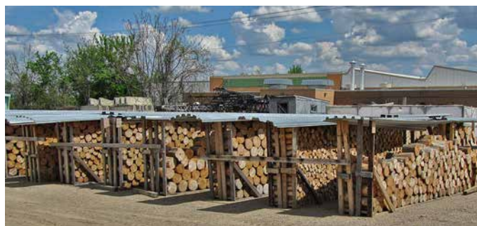
16.6. Logs cut to size, set in covered racks and sorted by log diameter. Credit: Studio Gang Architects.
