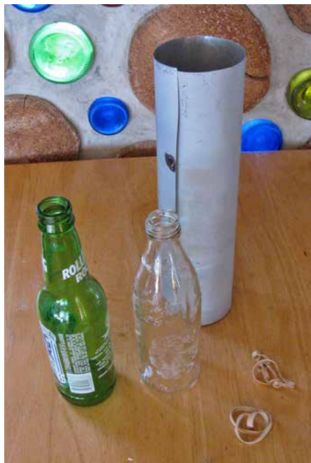
8.3. A green and a clear bottle of the same diameter can be plugged into a flexible cylinder and held fast with two strong elastic bands.
