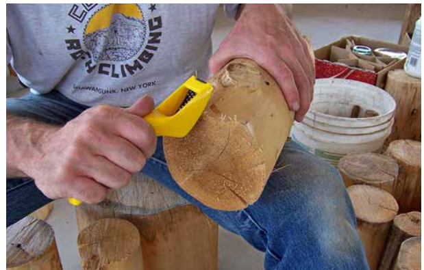
3.4. Holding the rasping surface of the scraper at a 45° angle to the log end, cut the little quarter-inch "hairs" off the edge of the log with a firm pulling motion.
