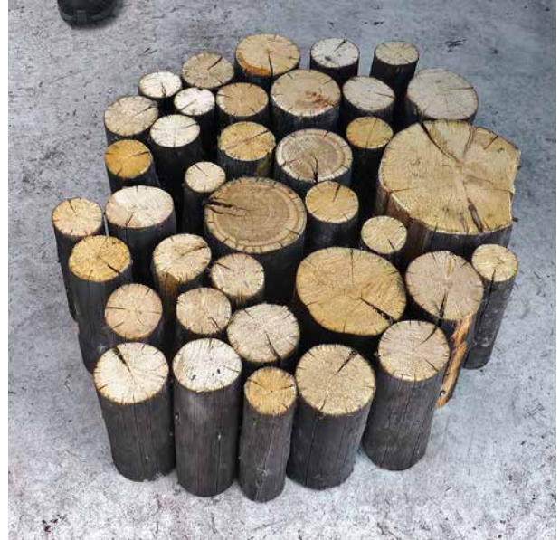
3.3. Any desired piece can be grabbed quickly if the log-ends are stored vertically near the work area.
