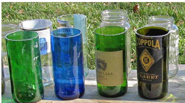
8.2. Bottles have been cut into tumblers (except for two jars, already useful), and are drying in the sun. When fully dry, they can be taped together.
