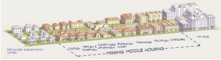
Fig. A.3 This diagram effectively illustrates how moderate density housing types can bridge the gap between single family detached and higher density elevator buildings. (Illustration © Opticos Design, Inc. Reprinted with permission)
