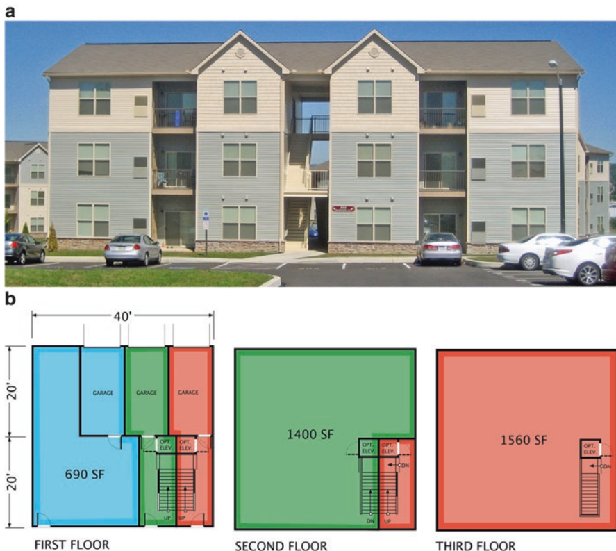
Fig. 8.8 (a) The very common three-story breezeway building combines open air circulation with surface parking to deliver affordable housing without elevators. (b) There are many variations of walk-up multifamily buildings; this example combines three units in a 40-ft square footprint and has integral garages
