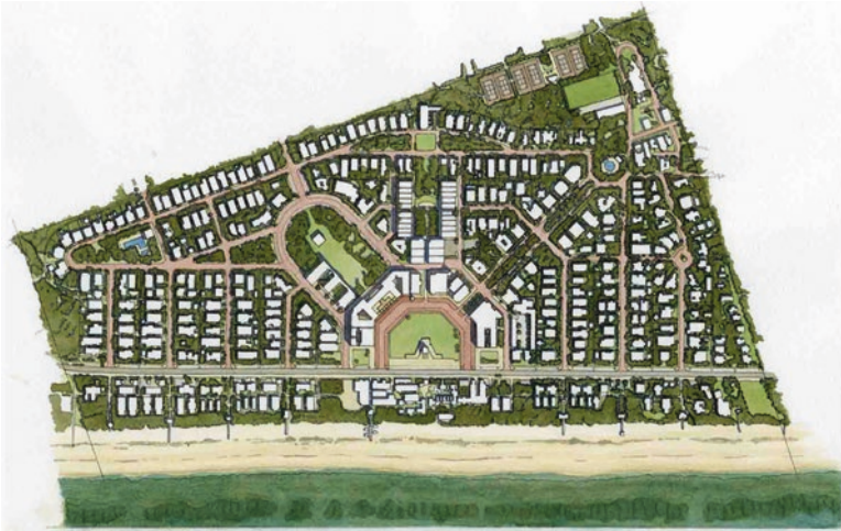
Fig. 2.11 DPZ’s plan for Seaside was inspired by the mixed-use, pedestrian-oriented coastal towns of the Southeastern US. The design formula included civic architecture and meaningful open spaces in key locations, traditional and sustainable building techniques, a regulating plan, and an urban design code. (Courtesy Duany Plater-Zyberk & Company)
