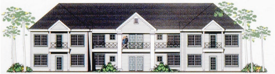
Fig. 8.6 The manor house concept may be appropriate at higher densities. This design for condominiums in South Carolina combines ten garden flats into a building intended to look like one larger dwelling. The central gable in the courtyard acts as a focal point for the overall building
