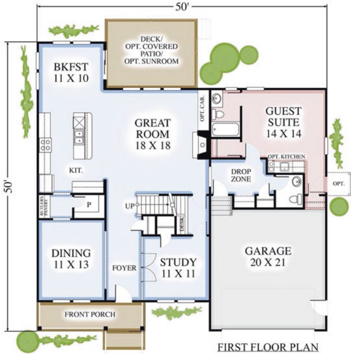
Fig. 5.13 Although most markets are dominated by four or five standard plan arrangements, new layouts such as the in-law suite plan are working their way into even the more design-conservative locales
