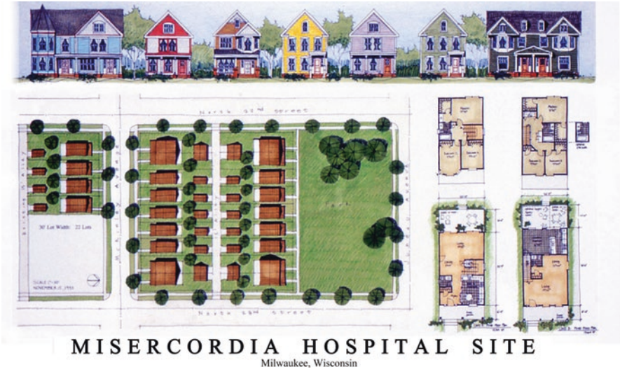
Fig. 4.16 Locating the garage in the rear of the lot, with access from an alley or lane, is a popular concept among traditionalist planners and based on historical precedents found in prewar communities
