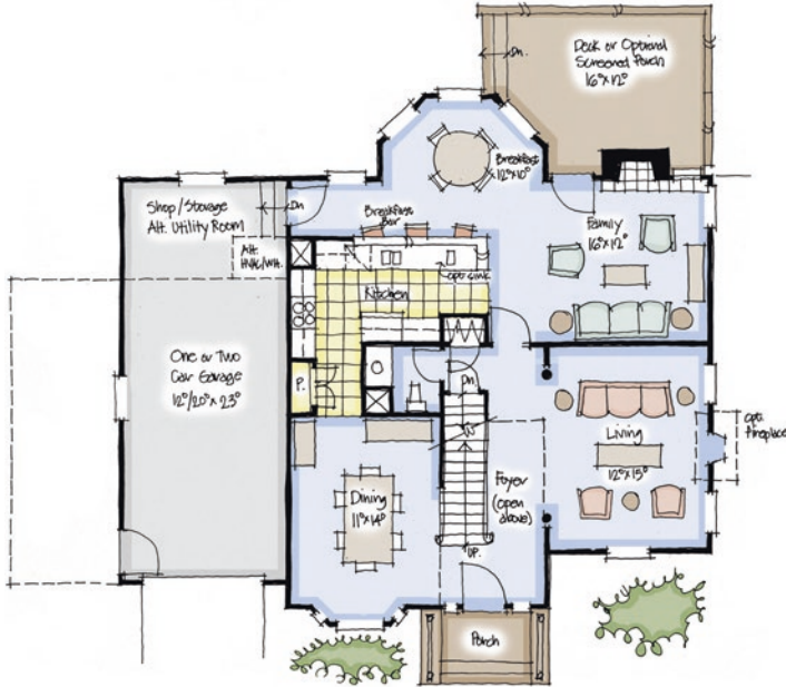
Fig. 5.22 One of the best ways to test the functionality of a plan is to furnish the rooms on paper. Curiously, this exercise is often overlooked in the design process
