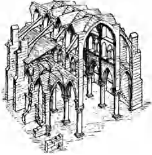
Gothic architecture showing construction of a Gothic church, illustrating principles of isolated supports and buttressing
