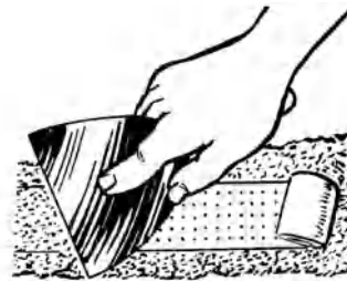
perforated tape covering a joint
