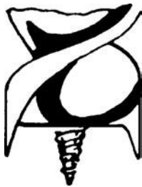
center bit showing cutting end
