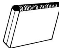
edge joint, 2 (welded)
