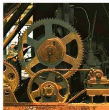
The gears used in the operation of a crane all rotate about fixed axes. Engineers must be able to relate their angular motions in order to properly design this gear system.
