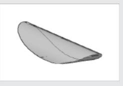
• An interference sphere marks the location of the interference. You can control its size and behavior in this box. Choosing Diameter by True Solid Extents limits the size of the sphere to the overlap of the interference, similar to the true interference solid.
