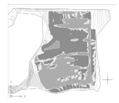
To show where large amounts of cut or fill could incur additional cost (such as compaction, or excavation protection), you would simply modify the analysis range as required.
