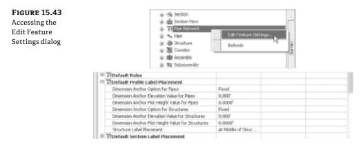
The Edit Feature Settings dialog has a cryptic batch of settings under Default Profile Label Placement. In a nutshell, these settings give your labels profile-view attachment points that you can customize. This section examines the structure labels closely. Note the default settings:
