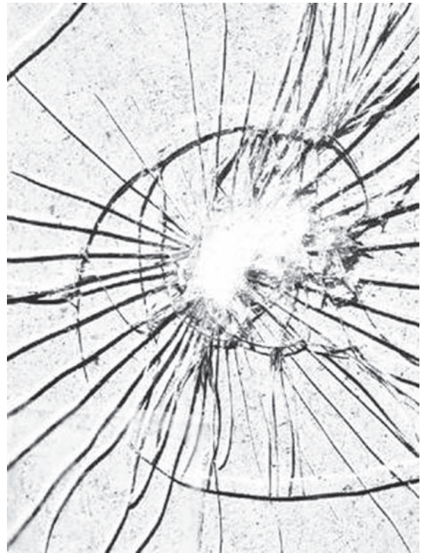
Fig. 58.4 Breakage pattern of laminated annealed glass.
