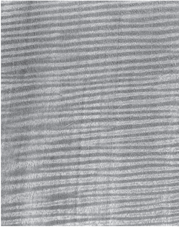
Fig. 52.18 'Fiddleback' figure on the longitudinal-tangential plane in Terminalia amazonia due to wavy grain development in the longitudinal-radial plane (© Building Research Establishment).
