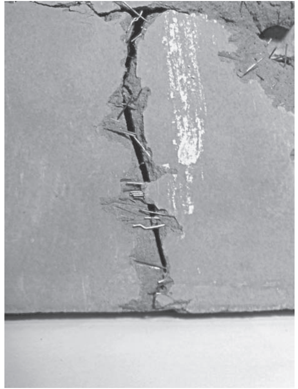
Fig. 48.4 Fibres bridging a crack in steel-FRC.
