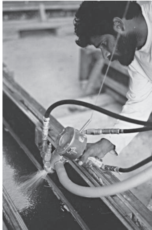
Fig. 49.3 Dual-spray concentric nozzle system for glass-FRC. The large pipe at the bottom right of the spray-gun supplies matrix; the small straight metal pipe at the top left is the roving intake. The black pipes supply compressed air both to power the roving chopper and to propel the chopped fibre and matrix. (Supplied by Iain D. Peter, Powersprays Ltd., UK ( www.power-sprays.co.uk ).)
