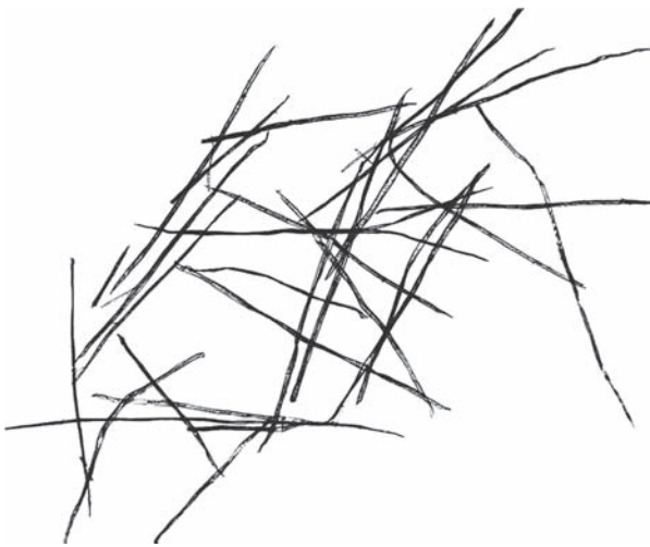
Fig. 52.7 Individual softwood cells (magnification × 12) (© Building Research Establishment).
