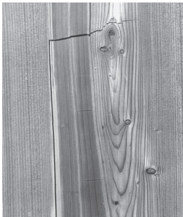
Fig. 52.16 A band of compression wood (centre left) in a Norway spruce plank, illustrating the darker appearance and higher longitudinal shrinkage of the reaction wood compared with the adjacent normal wood (© Building Research Establishment).
