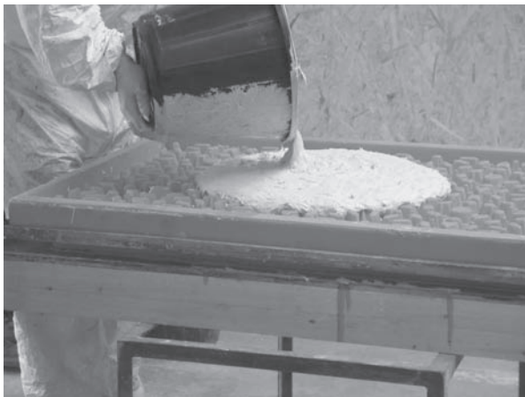
Fig. 49.1 Manufacture of a cast premix glass-FRC cladding panel. (Supplied by Iain D. Peter, Powersprays Ltd, UK ( www.power-sprays.co.uk ).)
