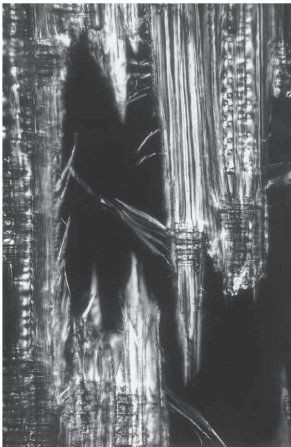
Fig. 54.8 Tensile failure in spruce ( Picea abies ) showing mainly transverse cross-wall failure of the earlywood (left) and longitudinal intra-wall shear failure of the latewood cells (right) (magnification \times 200 , polarized light) (© Building Research Establishment).
