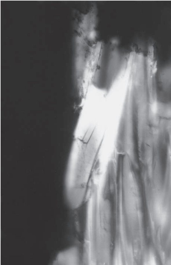
Fig. 54.11 Crack-stopping in a fractured rotor blade. The orientation of the secondary cracks corresponds to the microfibrillar orientation of the middle layer of the secondary cell wall (magnification \times 500 , polarized light) (© Building Research Establishment).
