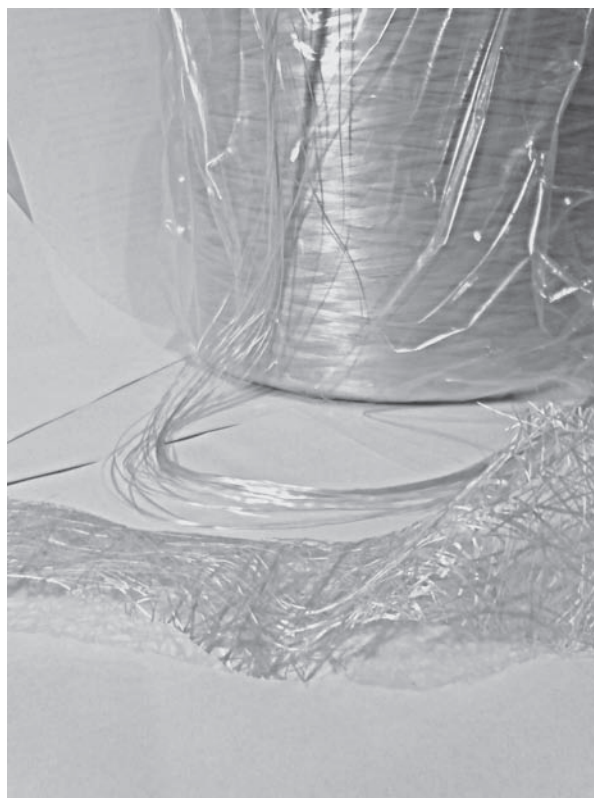
Fig. 45.4 Glass fibres for FRC. Foreground – chopped strand mat. Background – continuous roving for chopping.
