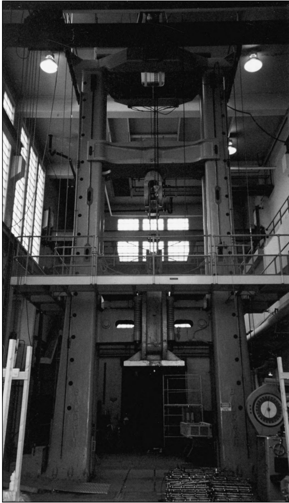
Figure 1.5 Three-story universal-testing machine, Seattle, Washington.
