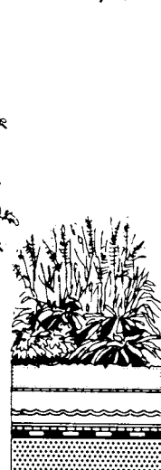
6 Zinco Floradrain roof cultivation system
