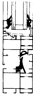
② As ① but with thermally separated profile sections (up to 37 dB)
