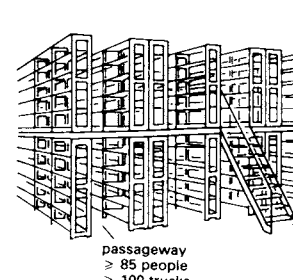
⑫ Shelving, one or two levels, made from units of wood or steel
