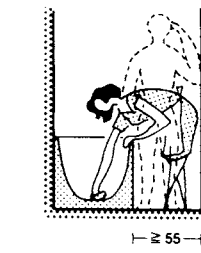
⑫ Minimum space between bath and wall
