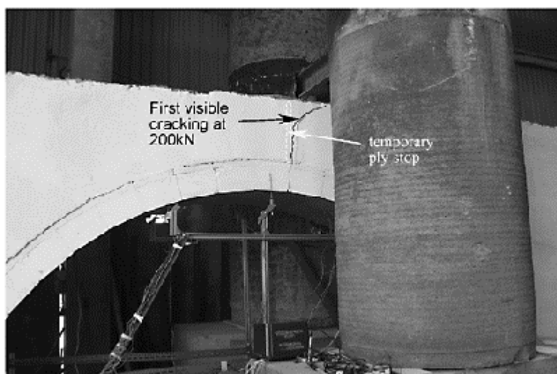
Figure 7. Full test load at third span at an applied load of 200kN.
