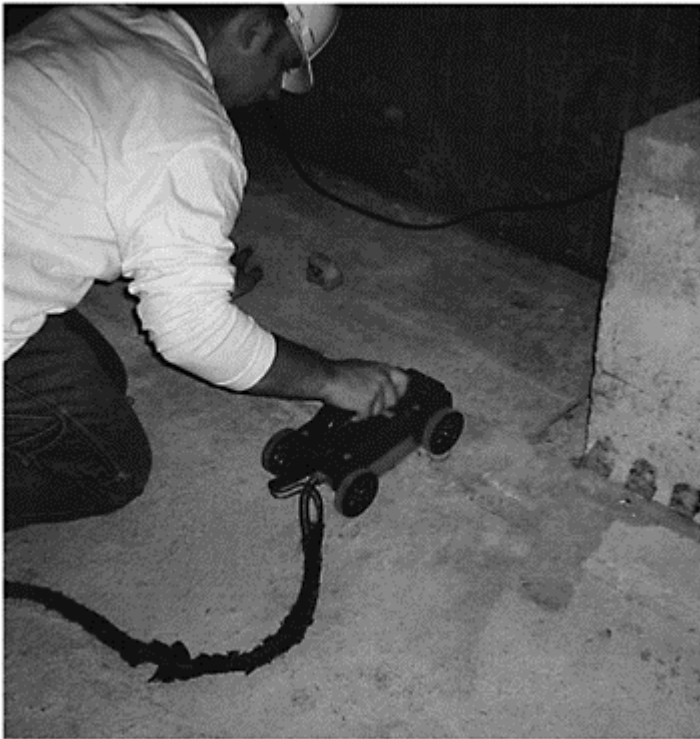
Figure 9. GPR investigation of box bottom slab using 1500Hz antenna.
