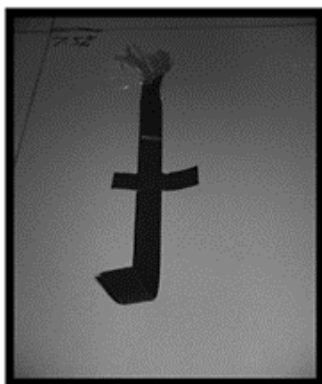
Figure 2. Typical failed specimen of polymer reinforcement.
