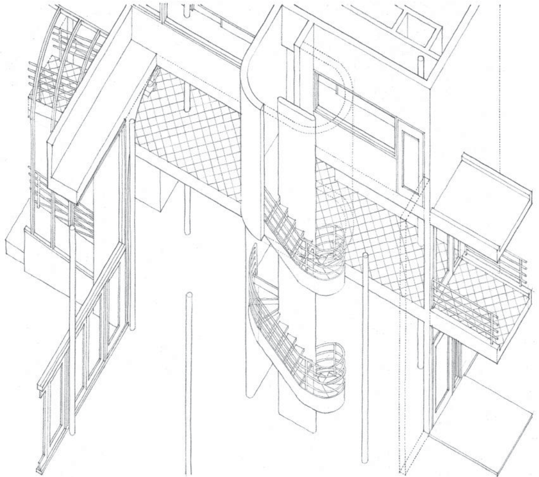
Plan oblique of living room stair, House in Old Westbury , New York, 1969–1971, Richard Meier
