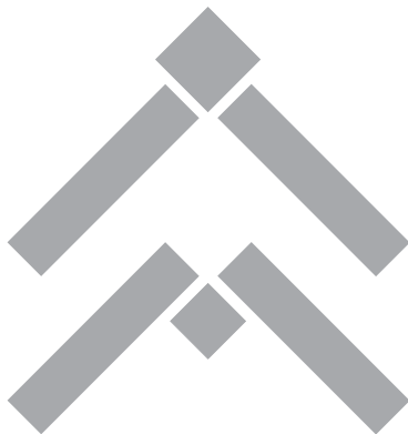
Corner Detail, Commonwealth Promenade Apartments , Chicago, 1953–1956, Mies van der Rohe. The corner member is recessed to be independent of the adjoining wall planes.
