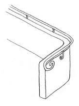
paratus. Opposing the possibility of allowing a detail to serve various functions is a strategy that separates its various tasks from one another, thereby clarifying them. A handrail, for example, may be set off from a concrete balustrade in order to distinguish clearly the functions of guarding against falls and providing a handhold.
