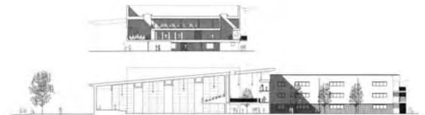
Section/elevation of main entrance and main hall showing upper level teaching and triple-height street
