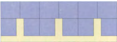
Diagram of break-out spaces in oversized single-loaded corridor
