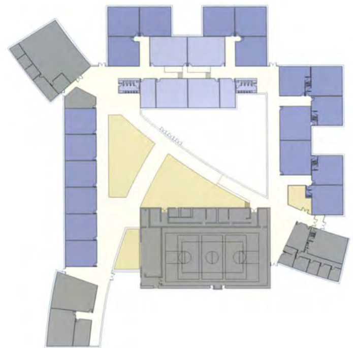
Plan showing public spaces at the key locations on the perimeter. Glenville Elementary School, Greenwich, Connecticut, Perkins Eastman Architects
