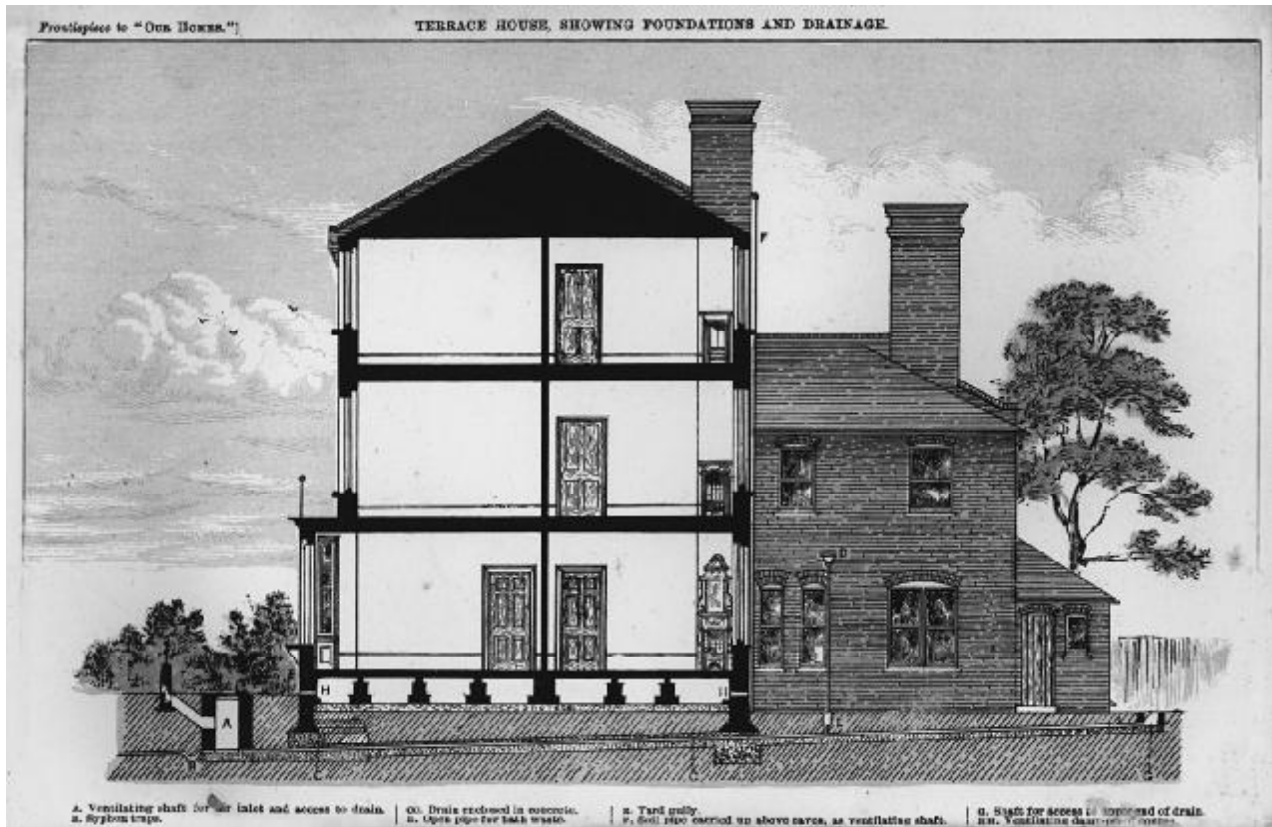
Figure 119 Terraced house, showing foundations and drainage.
