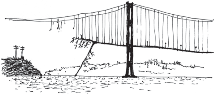
Tacoma Narrows Bridge in Washington State shortly after collapse due to rhythmic deflections caused by wind, November 1940. 4
