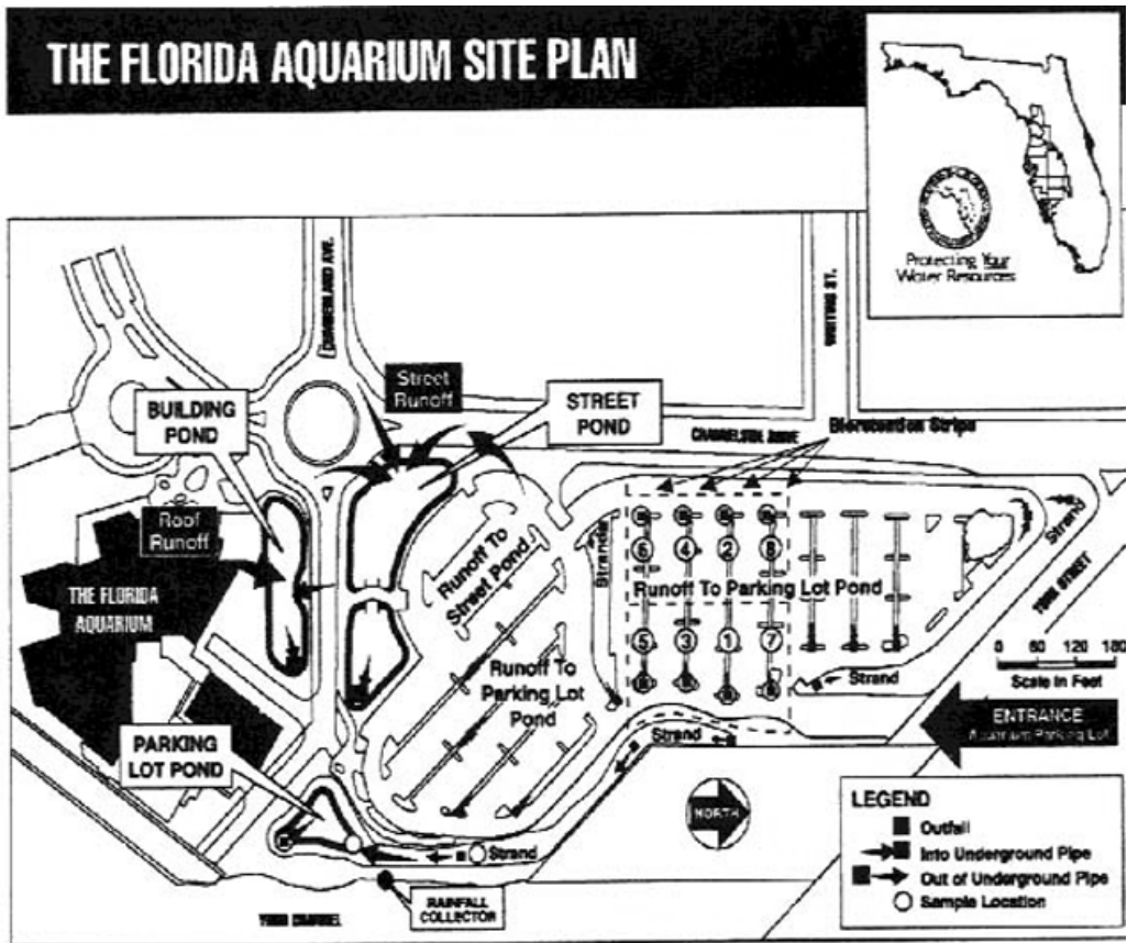
Figure I.15.12 The Florida Aquarium LID site features a treatment train approach that includes porous pavement, bioretention strips, and ponds. (Color version available at www.gsd.harvard.edu/watercolors . Password: lentic-lotic.)
