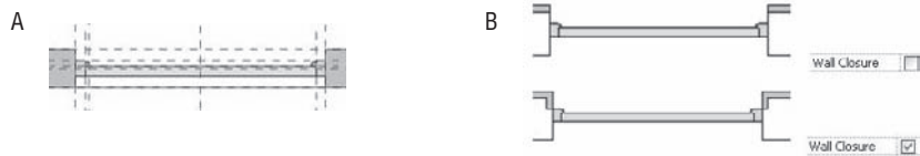
FIGURE 12.15 (A) The reference plane in the Family Editor, and (B) its effect when set to Wall Closure .
