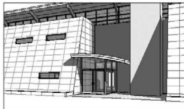
FIGURE 10.1 Revit design options used to explore alternative design solutions for an entry canopy.
