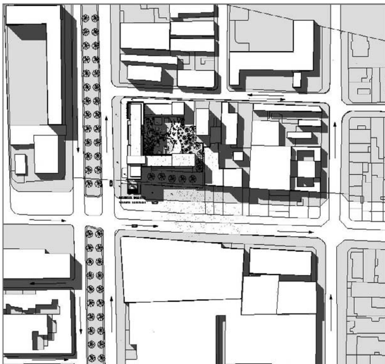
FIGURE 15.1 Analytical use of shadows in a site plan shows the effect of buildings on their environment.
