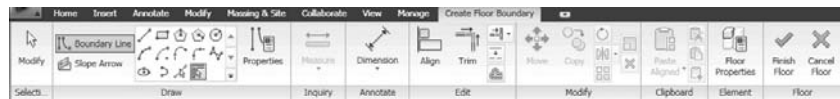
FIGURE 6.3 The Create Floor Boundary tab offers tools for sketching the floor shape.
