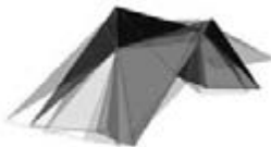
12.8 >Parametric model used to study folding sequences. Modifying the dimensions of the model manipulates the shape of the system. The formwork needed to pour the flat plate shapes can be generated on a variety of CNC tools, including lasers and routers.
