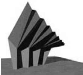
12.9 >Scale model of the cantilevering canopy: in the digital model each canopy segment was derived from a single generic parametric design object.
