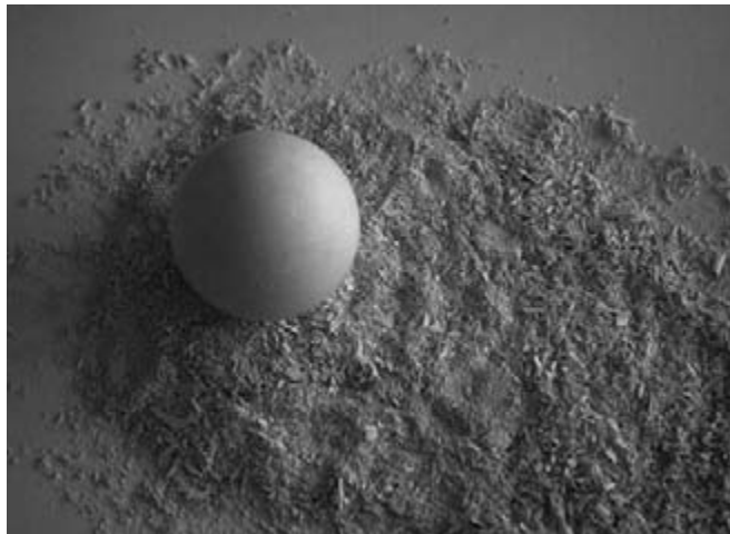
9.3 >Hand-turned plaster sphere with material removed during fabrication.
