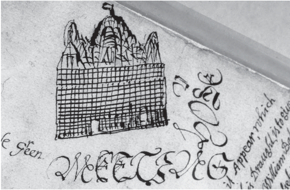
Figure 5.17. Detail, “. . . the foot way now in Contest.” View of the third meetinghouse in Ipswich, Massachusetts, drawn by a surveyor to contest a right-of-way claim in 1717. This meetinghouse was raised by Abraham Tilton and Abraham Perkins in 1699; its dimensions were 66 by 60 feet with 26-foot posts, the roof “with 2 [or] 3 gables on every side, with one Teer of Gallery round said house.” Courtesy of the Peabody Essex Museum, Salem, Massachusetts.
