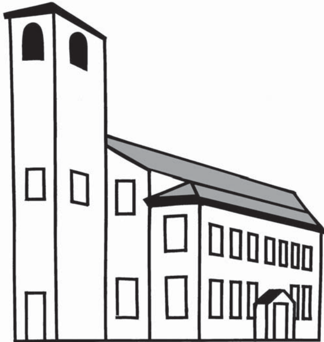
Figure 6.31. Schematic view of St. Peter's Church, Salem, Massachusetts, built 1733, seen from the southwest, showing the galleried lean-to on the long side added sometime in the late eighteenth century. Drawing by the author based on an 1833 watercolor by George A. Perkins at the Peabody Essex Museum.
