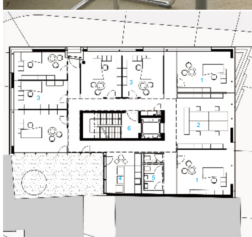
First Floor Plan (Left) 1. Office 2. Secretariat 3. Advisory Service 4. Kitchenette 5. Toilette 6. Circulation Core
