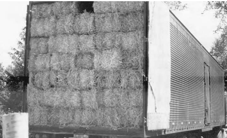
3.6: A transport trailer is a great way to move and store bales. The trailer can be rented and left on your site until you need the straw, eliminating one round of loading and unloading.
