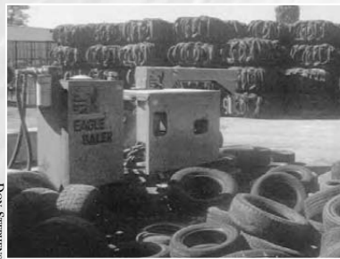
3.2e: Tire bales can make good foundations.
