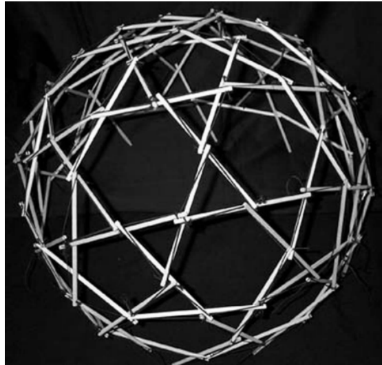
Fig. 8. "Circuit" model, tensegrity structure icosahedron Alt 4v
