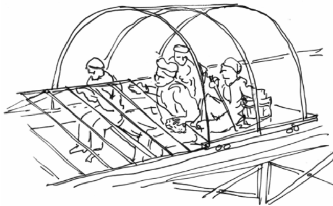
Fig. 7. Assembly of components of the Crystal Palace. a) Raising the arches; b) installation of the glazing
