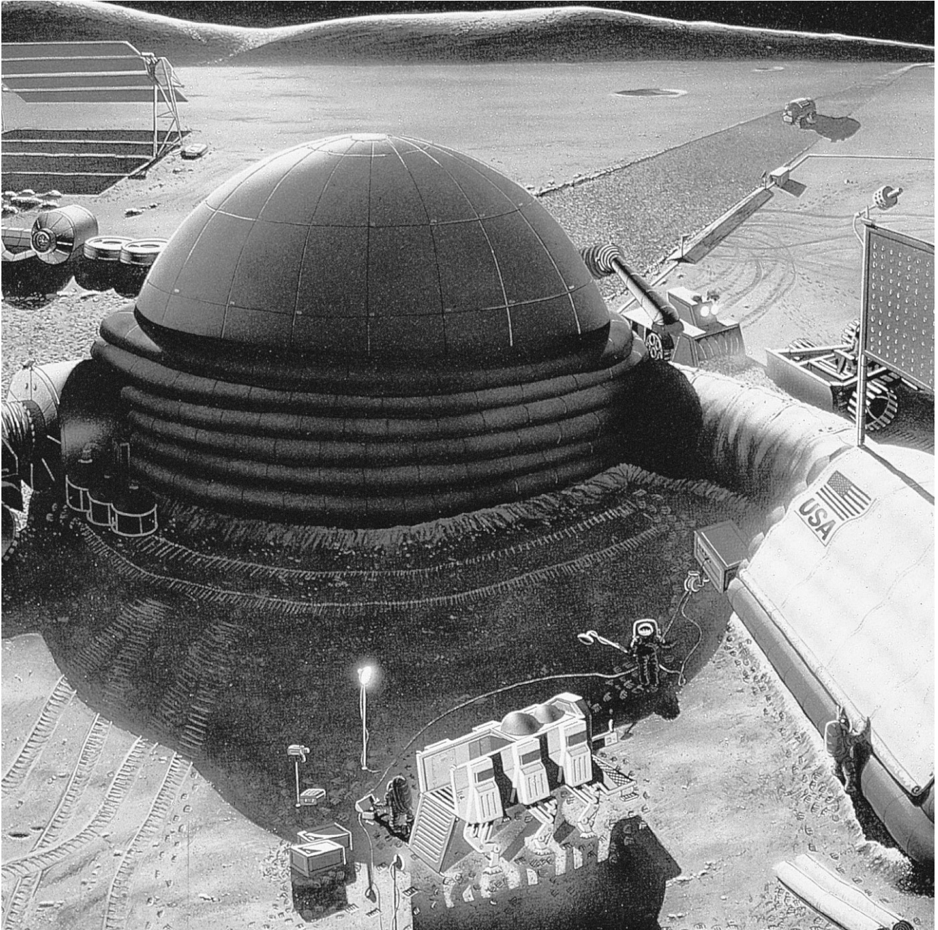
Fig. 15.2 NASA Lunar Outpost project, 1989. This early version of the inflatable habitat concept shows all the major components of a lunar base. At the centre is a spherical inflatable habitat built into the lunar surface and surrounded by a continuous bag of lunar regolith. To the top right is the graded road to the landing pad and top left is a solar power plant and oxygen production facility. Bottom right is a construction shack with thermal radiator on top.
