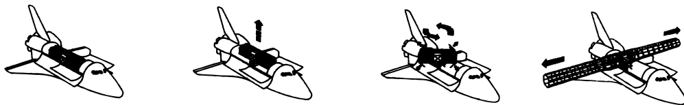
Fig. 3.1 Future Systems, Project 131, octagonal space beam system, 1985. A deployable octagonal structural beam system for use in space designed in conjunction with McDonnell Douglas Astronautics.
