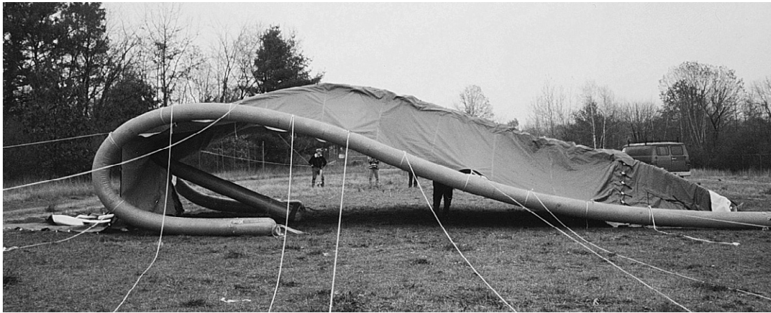
Fig. 12.26 LanMAS, test inflation of a prototype bay.
