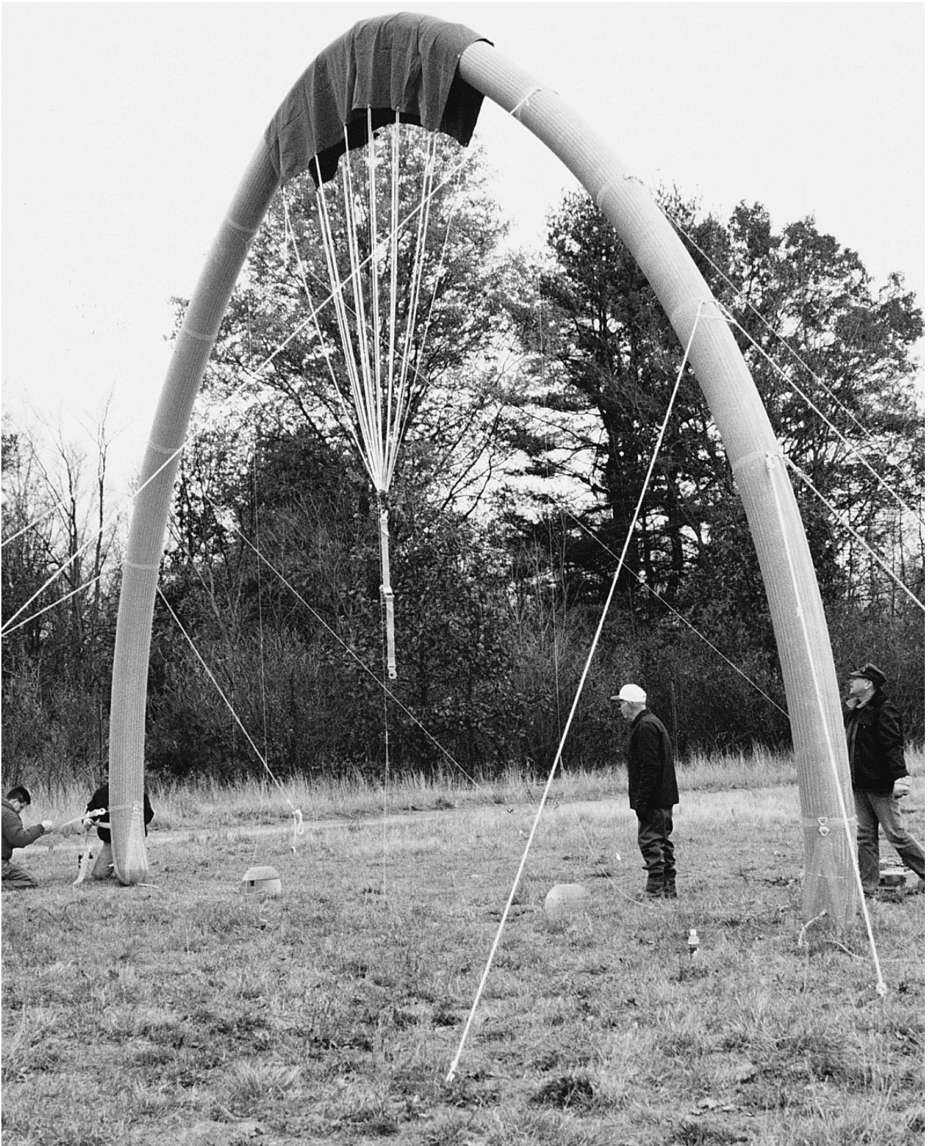
Fig. 12.22 LanMAS, small section arch prototype testing
