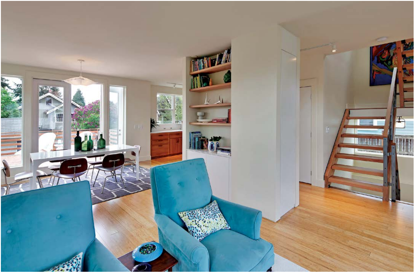
ABOVE: The flooring throughout the first floor is bamboo. A modification from the original plan, the open stair treads allow air and light to flow through the stairway.
