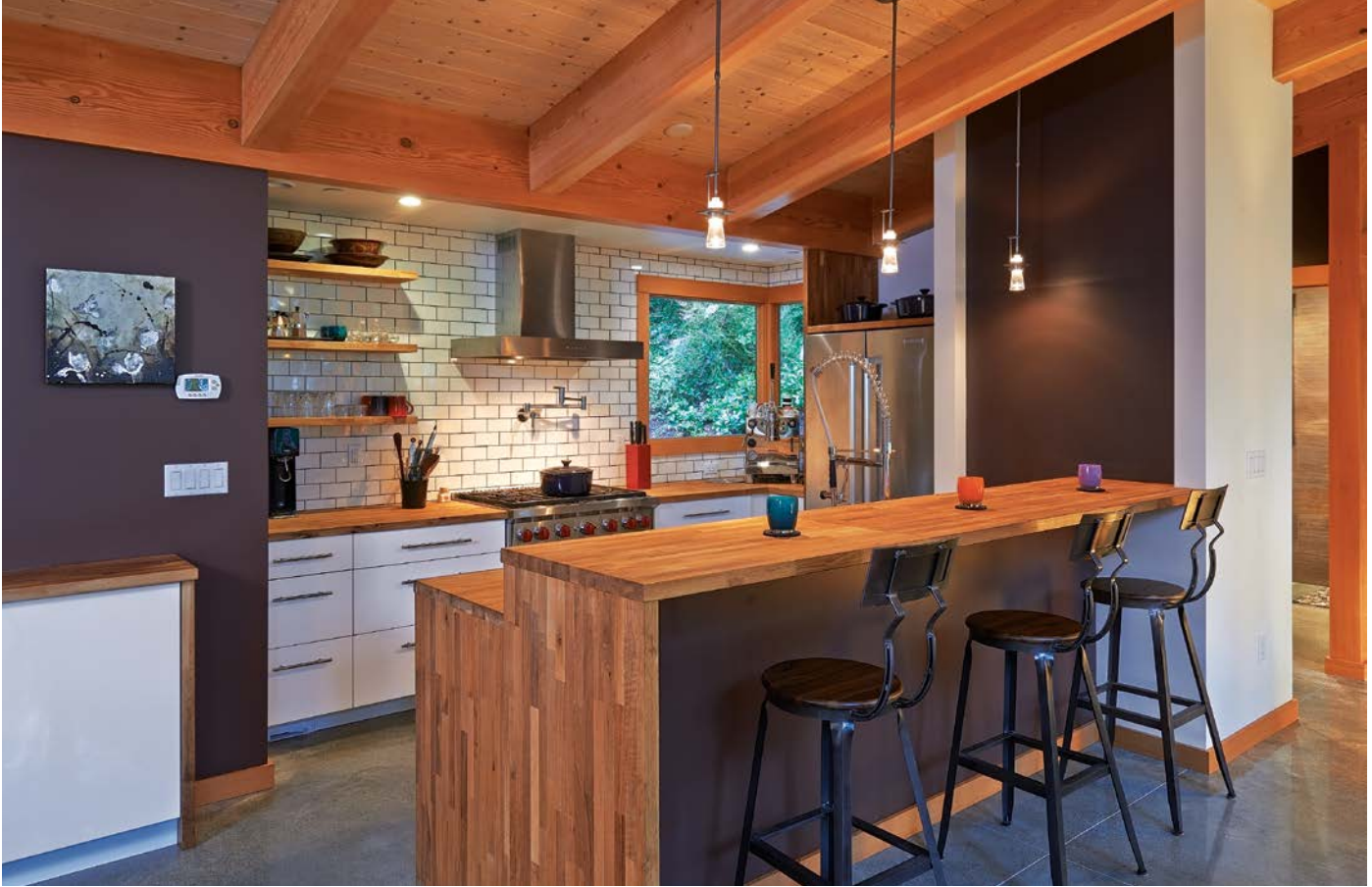
ABOVE: The white subway-tile backsplash and white cabinets contrast with the dark brown kitchen walls. Countertops are sturdy, long-lasting butcher block, while the floor is polished concrete with exposed aggregate to create a high-sheen reflective surface.
