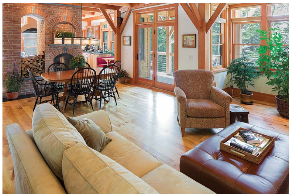
RIGHT: The masonry heater is in the middle of the open floor plan and can warm the whole first floor and the master suite above via a radiant floor panel on the second floor.
