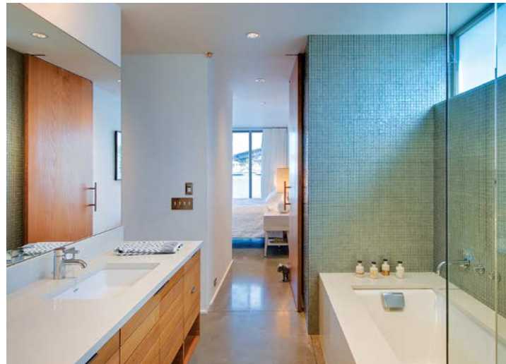
ABOVE: Radiant-heat concrete bathroom floors are a warm place to put cold feet in this simple but luxurious bathroom. The vanity cabinet is custom made of alder.
