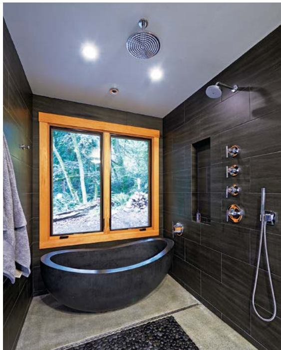
ABOVE: A sculptured black solid-stone bathtub and shower dominate one end of the master bathroom. Carved from a solid piece of granite, the tub fills from water cascading from a spout in the ceiling. Shower water drains through the river rock pebble mat in the floor. A separate rainwater showerhead provides a memorable showering experience.
