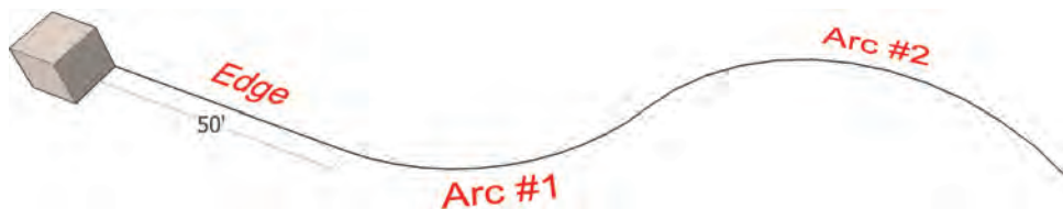
Fig. 8-8: Starting at the cube, draft a 50' -long edge and two arcs as indicated.
