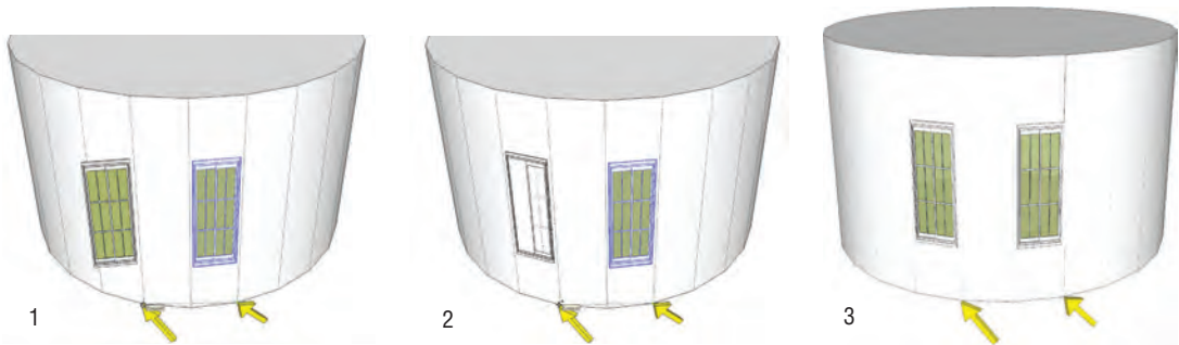
Fig. 11-6: A Window component being copied from one cylinder face to another using endpoints of edges for reference (1). Copied component correctly affixed to destination face (2). Once placed, the window will cut a hole in cylinder face (3).
