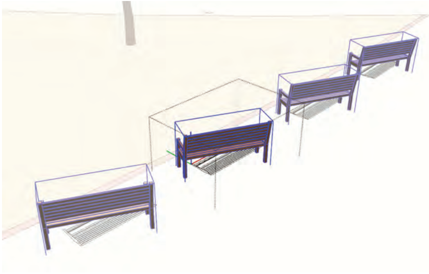
Fig. 19-15: The inserted 3D Bench component. The 3D component needs to be rotated and adjusted to face the correct direction. To universally adjust all of the benches, do this while you are working in the component instance.
