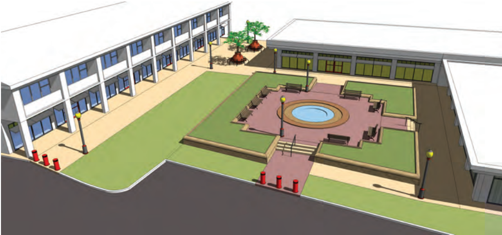
Fig. 10-13: Import and insert custom-made site components from Chapter 8. Insert the bollards, pedestrian lights, park bench, planter bench, and hand rail.
