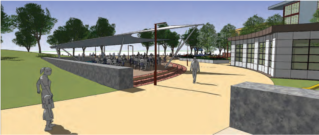
Fig. 19-59: By including people, you provide important scale that helps define the sizes, shapes, and relationships of the various site details and objects.
