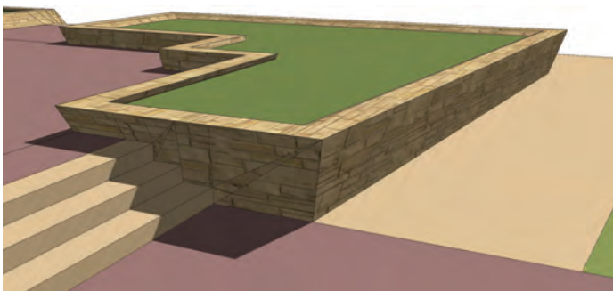
Fig. 7-50: The levered vertical faces of the wall
