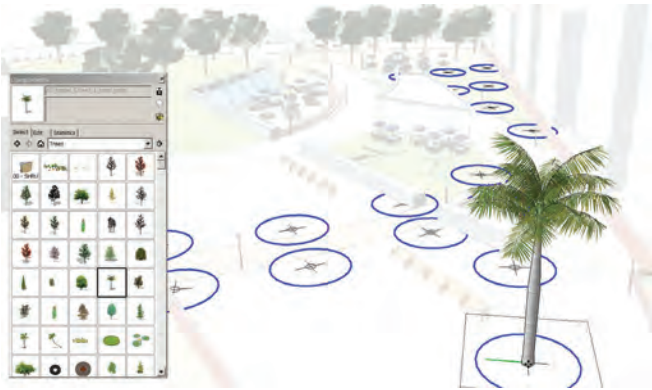
Fig. 19-22: A 3D Palm Tree component inserted directly into the Tree 2 component instance
