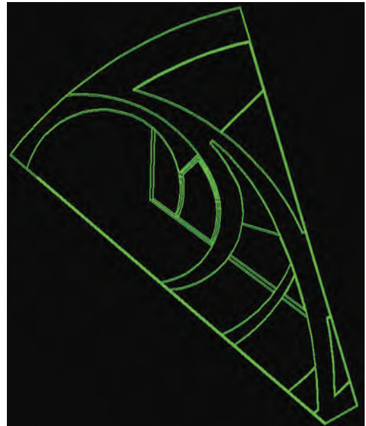
Fig. 16-5: The Flatwork Base linework is organized into an AutoCAD base file. This is the first file with lines that is imported into SketchUp.
