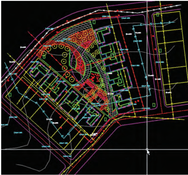
Fig. 16-1: An AutoCAD base file filled with the relevant project information: architecture, civil, utility, survey info, and the site plan
