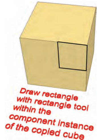
Fig. 3-5: In the component instance, draw a rectangle on the cube face as indicated.
