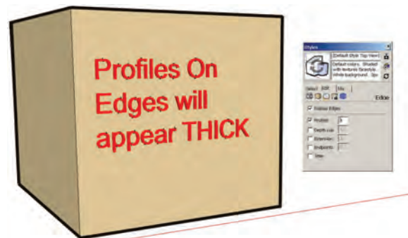
Fig. 2-21: Profiles are checked "on," displaying thicker edges.
