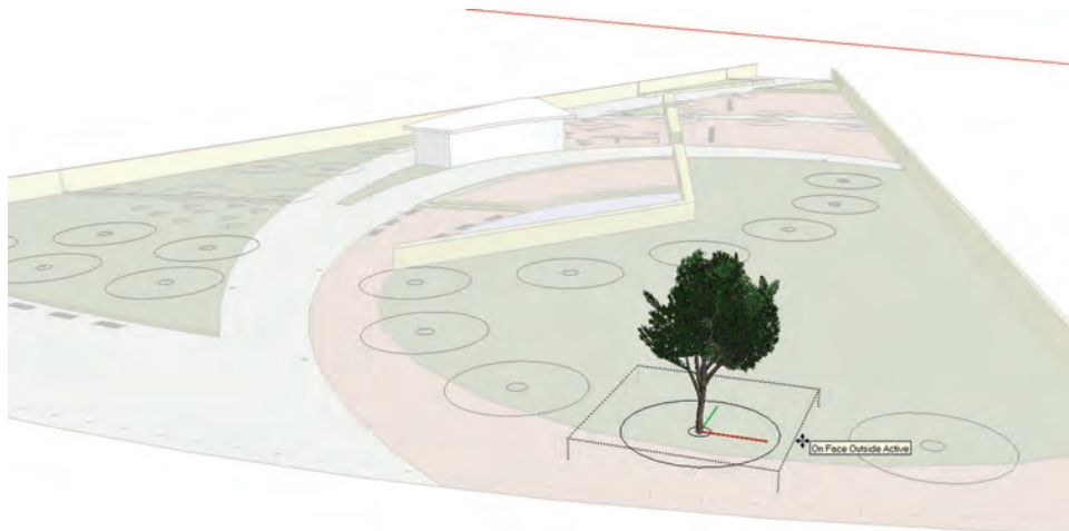
Fig. 16-12: Editing the 2D block/component and pasting a 3D component into the block is a quick way to add detailed elements to a model.
