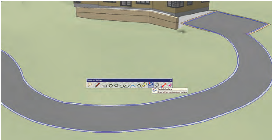
Fig. 15-32: Using Tools on Surface's Offset tool, select the road and offset a 6" curb.
