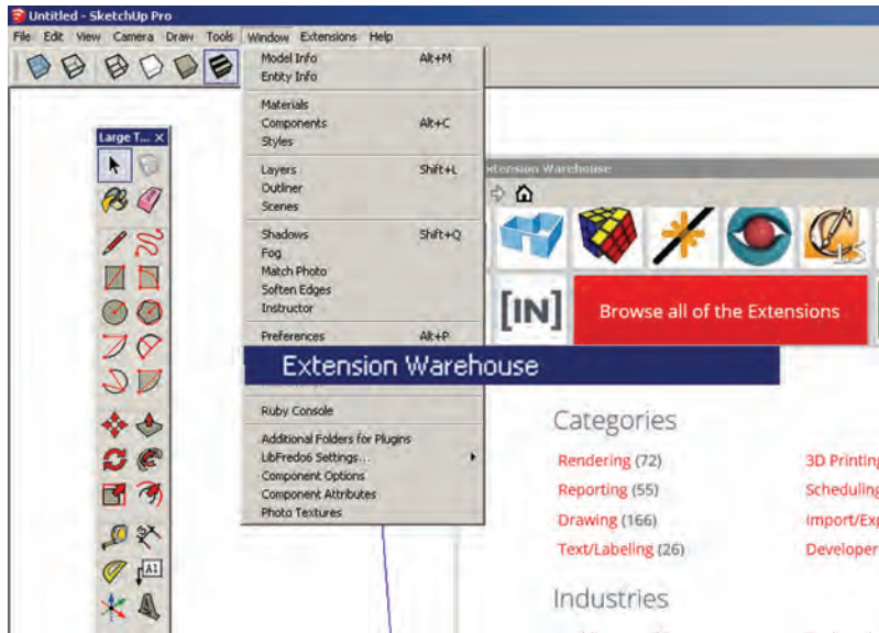
Fig. 5-5: In the Window menu, select Extension Warehouse to open the Extension Warehouse browser.
