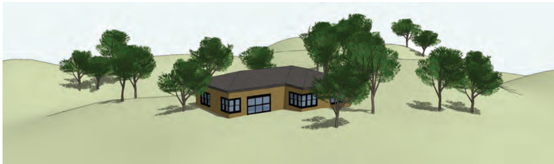
Fig. 12-25: Components land on the terrain at the first face they intersect downward along the vertical axis. The result is that the components “hug” the terrain model. This is easier than trying to place each component on a specific surface location on the terrain.
