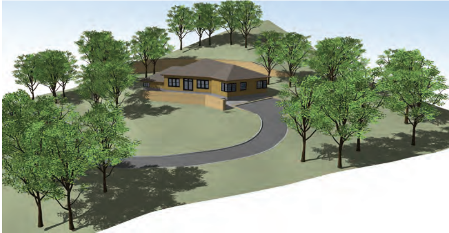
Fig. 15-36: Replace the 2D blocks with 3D trees. Use CLF Rotate and Scale Multiple on the vegetation. Turn on the shadows and export the scene.
