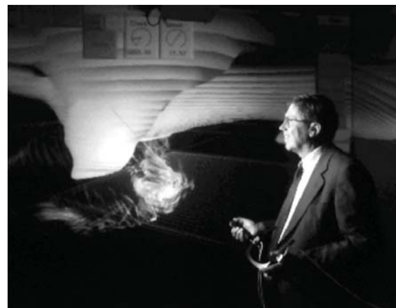
3.8: Enabling researchers to engage information in ways previously unavailable, the Cave provides an immersive virtual-reality room for visualizing and engaging spatial environments as they play out scenarios in front of you. See http://cave.ncsa.uiuc.edu
