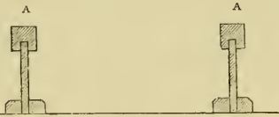
FIG. 22.—SECTION OF BOX OR PIT OF THEATRE. The tops of the partitions (A A) form the Aisles.
