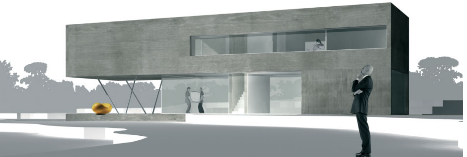
Maria Giuseppina Grasso Cannizzo, MFS House, Syracuse, Sicily, 2006 The shape comes from a prismatic reinforced concrete monolith from which some parts have been cut off. On the ground floor there is a glass volume and a porch, and the upper floor hosts an open-air space for meditation.
