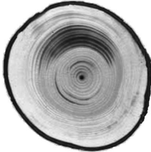
Fig. 1.2. Compression wood (dark patch).
