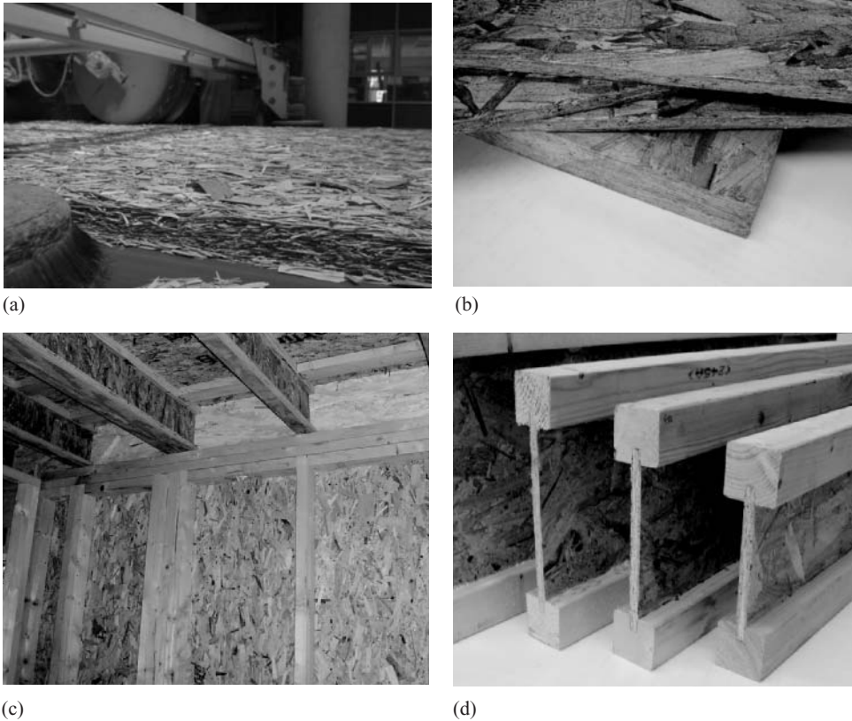
Fig. 1.14. OSB: (a) production before the press (photo courtesy of Wikipedia Foundation); (b) and (c) OSB boards and wall panels; (d) OSB webs in I-joists.
