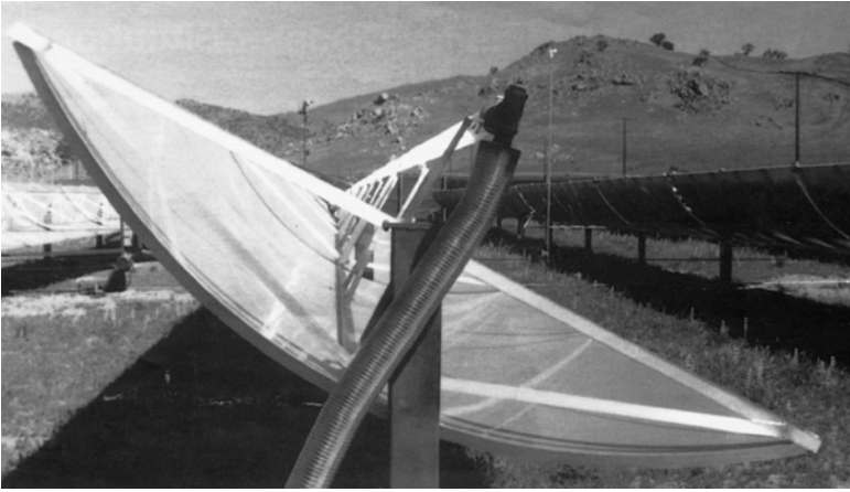
Figure 2.16 Solar thermal parabolic trough collector (courtesy of Caddet)
