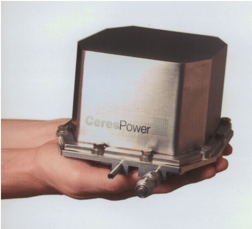
Figure 7.5 Micro-fuel cell by Ceres Power (courtesy of Ceres Power, www.cerespower.com )
