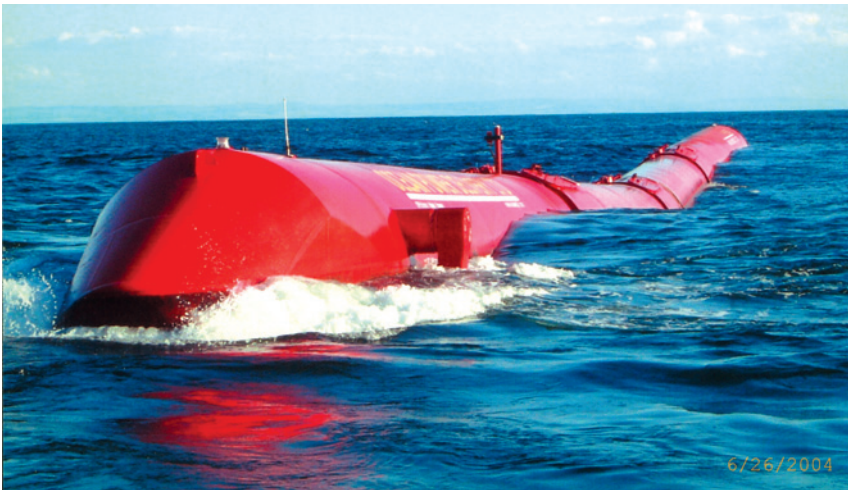
Figure 11.6 The Pelamis demonstration machine (courtesy of Ocean Power Delivery Ltd)
