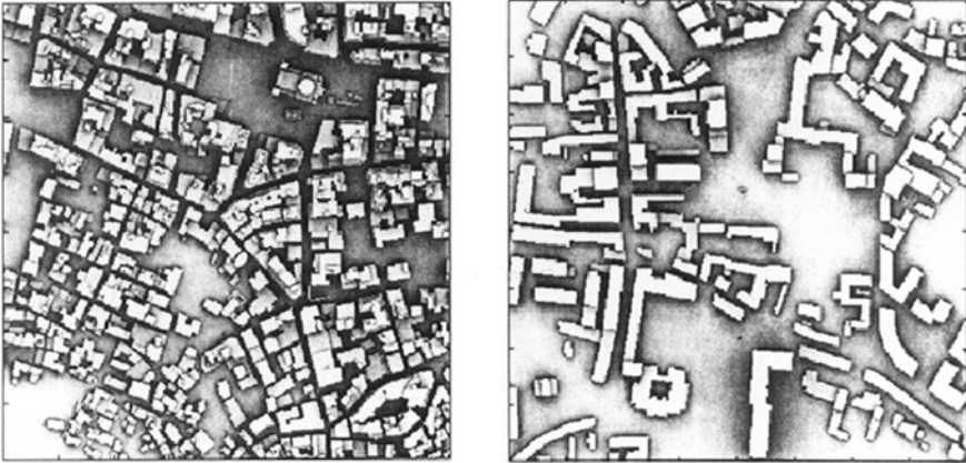
Figure 6.4 Sky view factor for two towns: medieval Athens (left) and Grugliasco, Italy (source: The Martin Centre, Cambridge)
