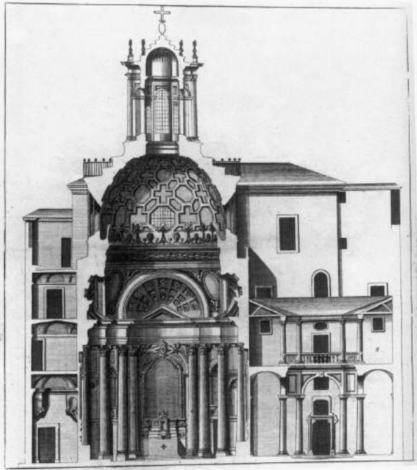
FIGURE 2.2 Francesco Borromini – San Carlo alle Quattro Fontane (1638–41), Rome. Engraving showing section through the church, by Sebastiano Giannini (c. 1730). Wikimedia Commons.
