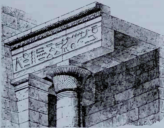
Anta extending the architrave above a row of columns up to the sloping front of a pylon
