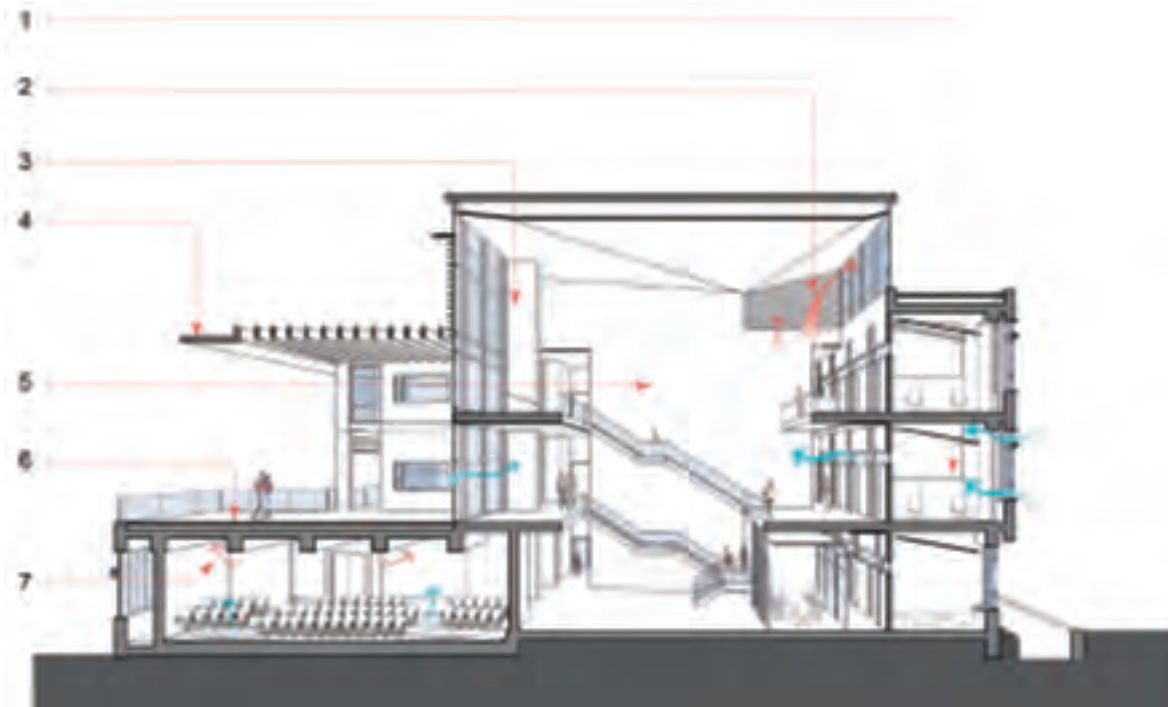
The multi-level atrium boosts natural ventilation for surrounding offices.
