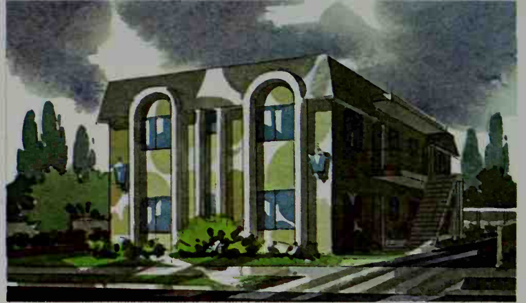
Start the shades and shadows on the building and put in the basic building washes.
