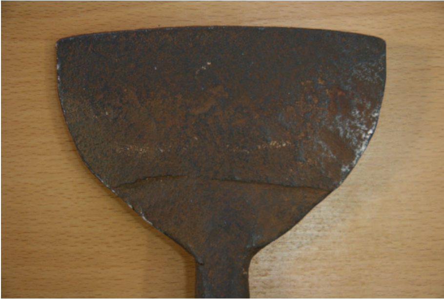
Figure 32 Welded edges on Brick Axe B. (Courtesy of Jay Close)
