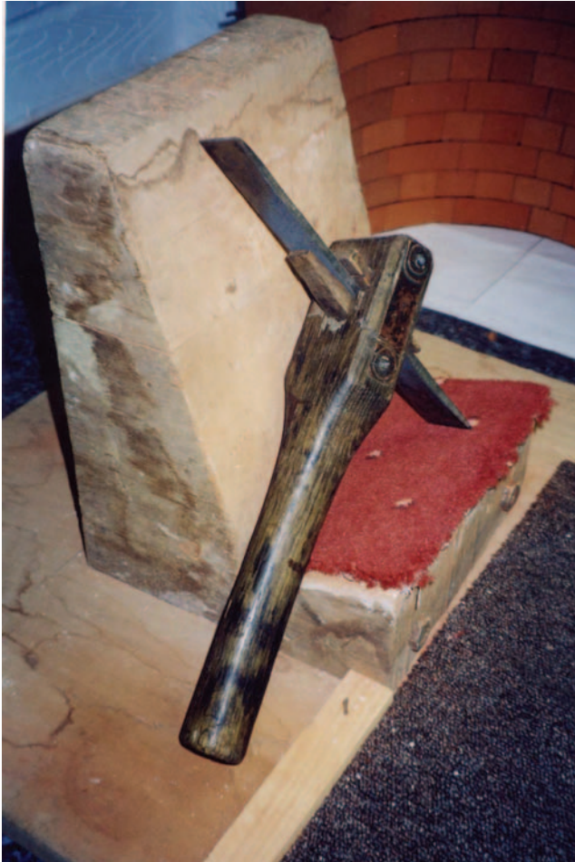
Figure 128 Bricklayer's Scotch resting against a cutting block.
