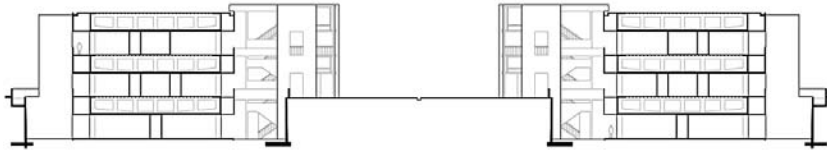
9.3 North-south section through laboratories and service floors. Salk Institute for Biological Studies, La Jolla, CA, 1959-1965. Architect: Louis I. Kahn. Drawing by A. B. Dixon
