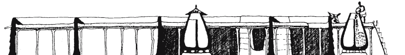
FIG. 44 : PART PLAN OF AND SECTION THROUGH A LOBI HOUSE (FROM THE NAKORI STUDY, DEPT. OF ARCHITECTURE, U.S.T., 1974)
