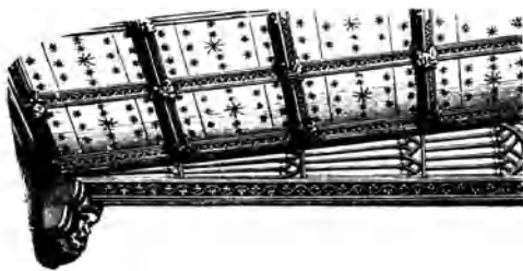
ribs, 2 dividing a ceiling into squares
