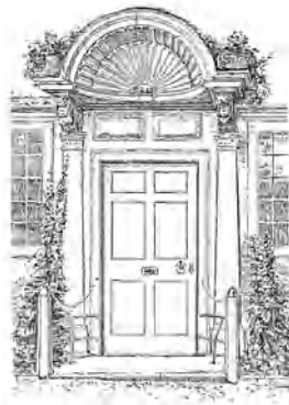
bracketed hood above a door
