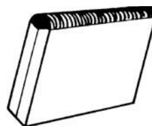
edge joint, 2 (welded)
