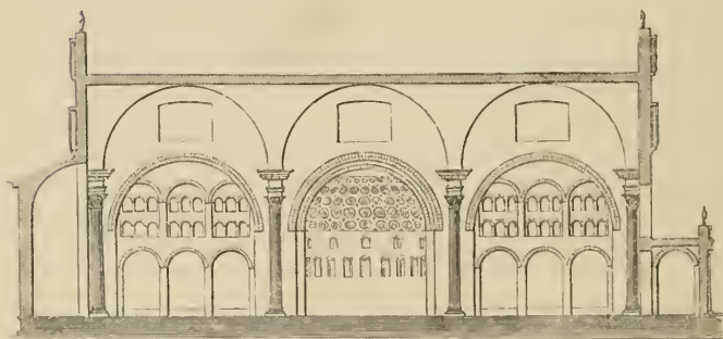
Longitudinal Section of Basilica of Maxentius. Scale 100 ft. to 1 in.
