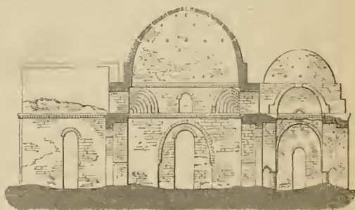
304. Section on line A B of Palace at Serbistan. From a drawing in Flandin and Coste's Voyage en Perse . Scale 50 ft. to 1 in.
