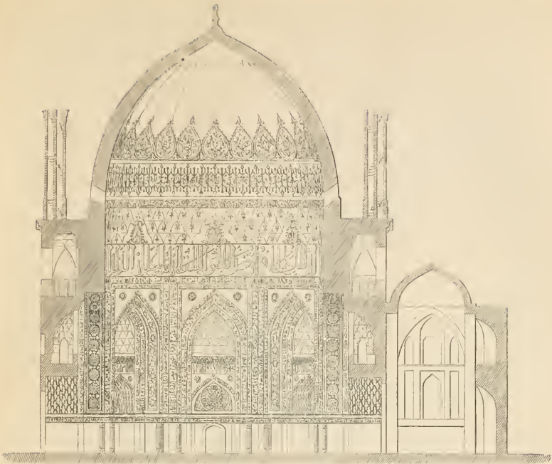
328. Section of the Tomb of Sultan Khodabendah at Sultanieh. From Texier's Arménie et la Perse . Scale 50 ft. to 1 in.
