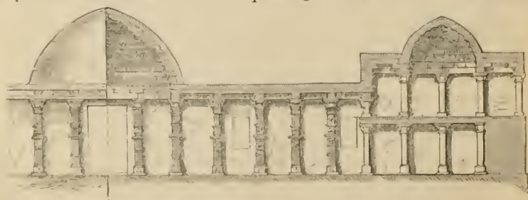
336. Section of part of East Colonnade at the Kootub, Old Delhi. Scale 25 ft. to 1 in.
