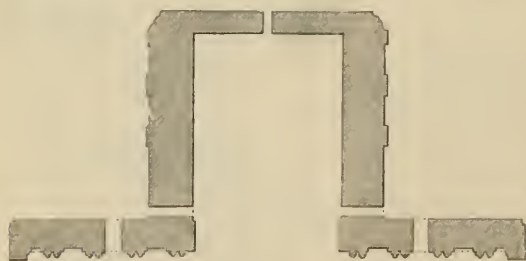
308. Plan of Tāk Kesra at Ctesiphon. From Flandin and Coste. Scale 100 ft. to 1 in.
