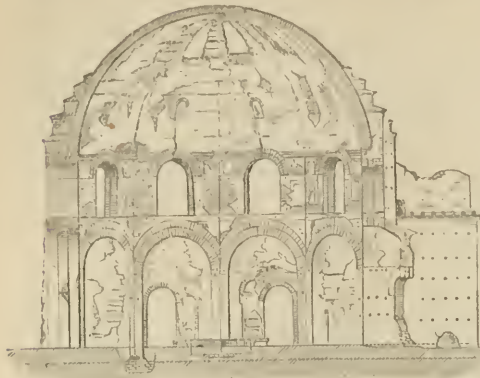
284. Section of Minerva Medica. Scale, 50 ft. to 1 in.
