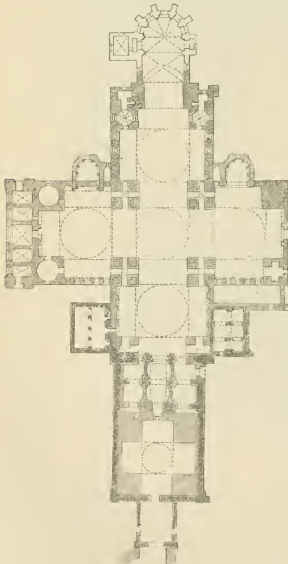
486. Plan of St. Front, Perigeux. From F. de Verneilh, Architecture Byzantine en France . Scale 100 ft. to 1 in.
