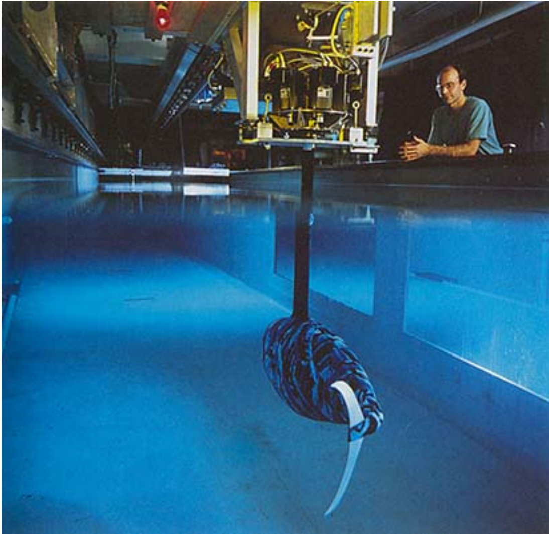
Plate 3 Robot tuna hanging from carriage in Ocean Engineering Testing Tank Facility at MIT. Source: Triantafyllou and Triantafyllou 1995. Photograph by Sam Ogden; used by courtesy of Sam Ogden and with permission of Scientific American, Inc.
