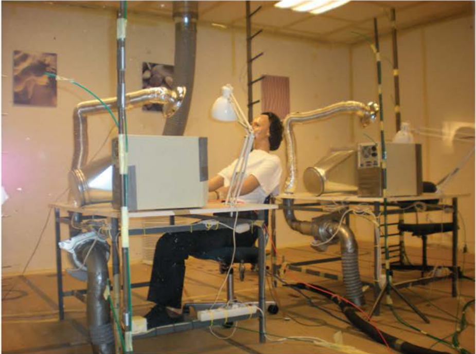
Plate 23. Indoor climate chamber. Source: Danish Technical University Indoor Climate Research Unit.
