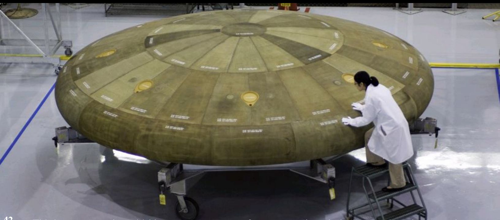
This is a prototype heat shield to protect astronauts from extreme heat during re-entry into the atmosphere.
