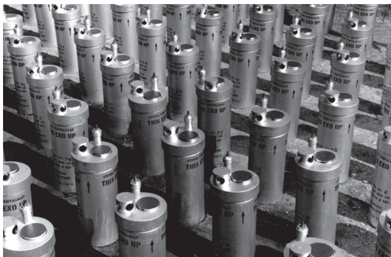
200-pound solid fuel JATO cannisters, the invention of John Parsons, as produced for Allied use in World War II.
