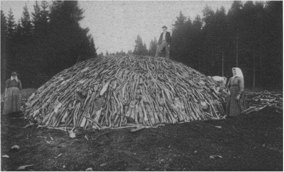
Figure 151: photo of typical turn of the century charcoal burners at work, an earth covering over such a woodpile would be used to limit the oxygen supply to the wood, causing a more uniform change into charcoal. Without such an earth cover, it would all burn away into ashes as a big bonfire.
