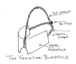
An additional strap is affixed to the blindfold, designed to go over the top of the head. It is attached to the elastic strap at the rear of the headband, where a large button is affixed.
