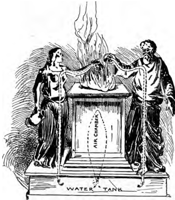
HOW THE STATUES WERE MADE TO POUR LIBATIONS WHEN A FIRE WAS KINDLED ON THE ALTAR.
