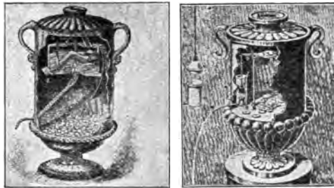
A RECENTLY PATENTED SLOT MACHINE ALMOST IDENTICAL WITH HERON'S WATER-VESSEL
