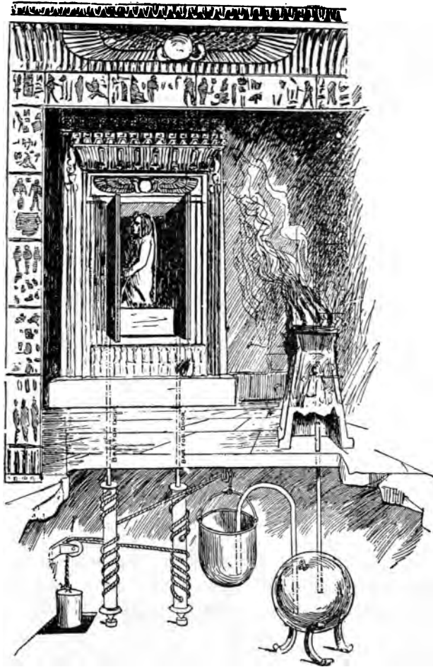
MECHANISM WHICH CAUSED THE TEMPLE DOORS TO OPEN WHEN A FIRE WAS LIGHTED ON THE ALTAR.
