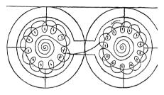
and fastened so that as it unwinds in one of the boxes it winds up the other in the second box. The clock is wound once a day, and as the running down of one of the spiral coils winds up the other the latter serves to run the clock during the night. Though it was described with much detail the mechanical working of it was not made clear, and hence we can only mention the mgenuity of the subconsciousness in constructing a plausible piece of machinery.
